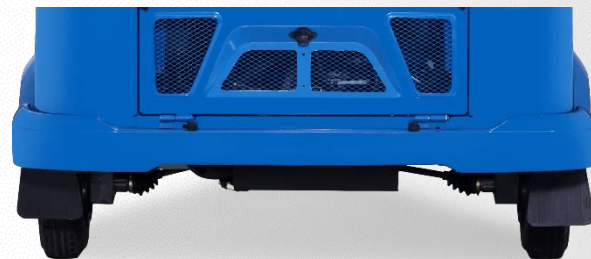
Rigid chassis mounted bumper
