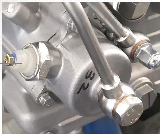
OIL PRESSURE SWITCH ON THE ENGINE
