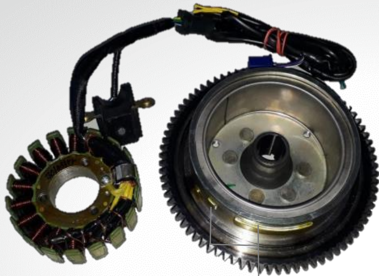
Dual-pip on the rotor circumference
