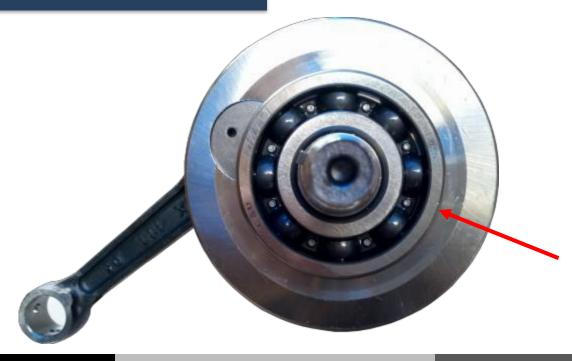
Feature: Crank shaft ball bearing
