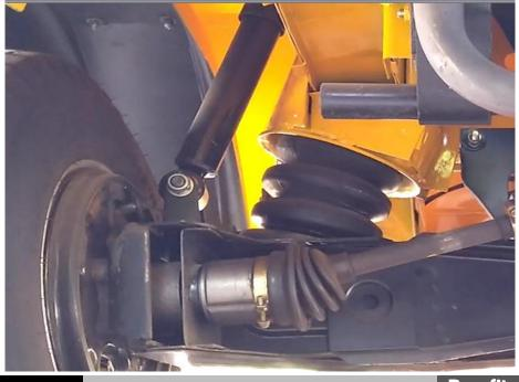
Feature: Rear Suspension (Rubber spring with hydraulic shock absorber)
